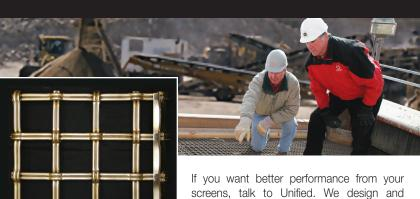
Like our **new TwinWire screen media:** Customers wanted a high-impact, top deck, wire cloth screen with maximum open area. The Unified team designed and manufactured TwinWire screens to ensure uniform openings with a strong lock-crimp construction. In field tests, a 2" opening with a 3/8"-diameter TwinWire screen outperformed a 5/8" single-wire screen.
