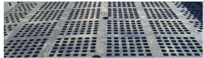
Rubber and wire cloth screen deck with rubber side tension rails
