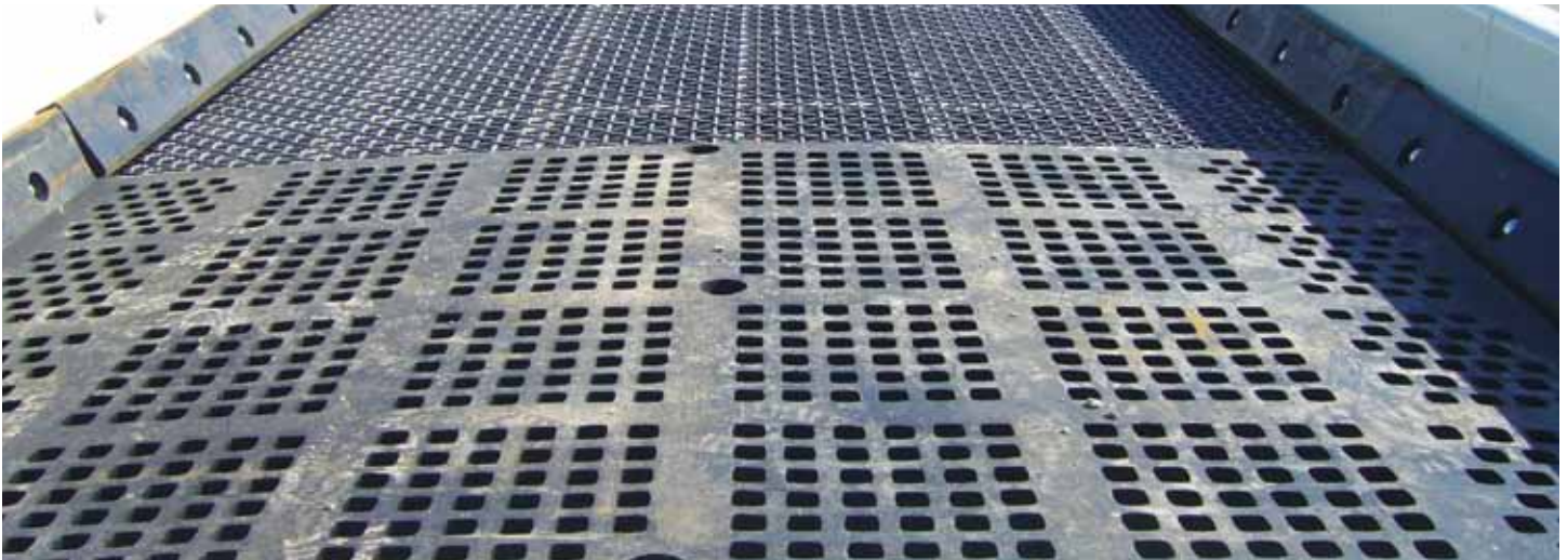
Rubber and wire cloth screen deck with rubber side tension rails
