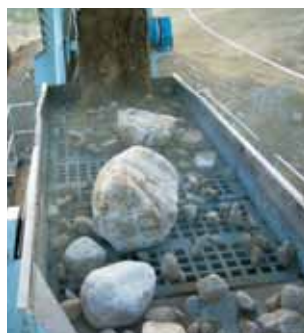
Rubber Grizzly Screens for high impact at the feed end of the deck. Note: Center boulder weighs 3 tons.
