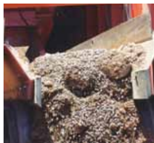
Discharge end of belts showing end of Rubber Canoe Liners
