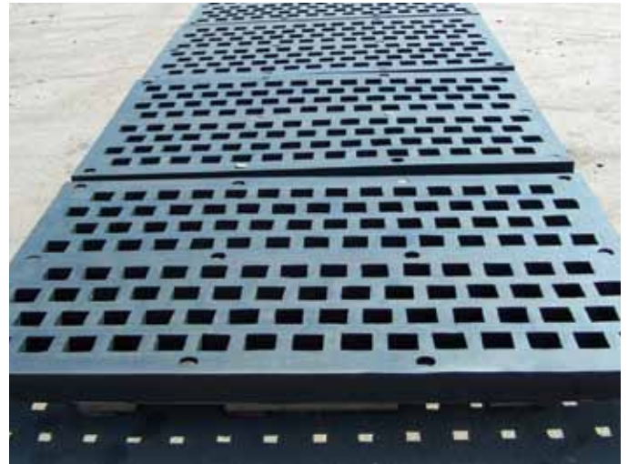
Bolt down rubber-clad punch plate in 4' x 6' panels
