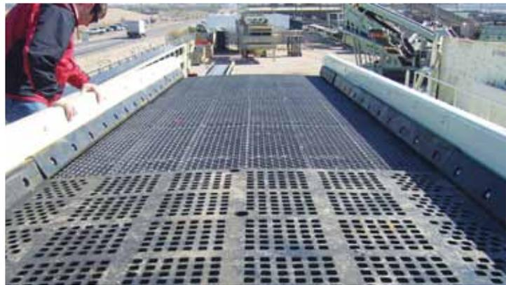
*Rubber and Wire Cloth Screen Deck with Rubber Tension Rails*
