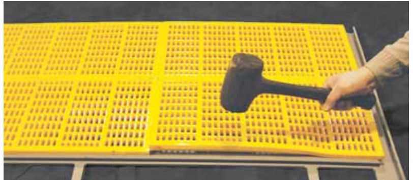
The replaceable FLOWMAX modular tension frame with polyurethane modules.
