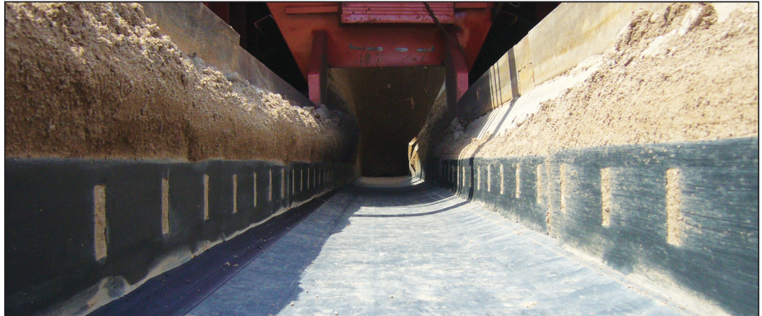
Belt Feeder with Canoe Liners on either side shown after 6 months of wear.
