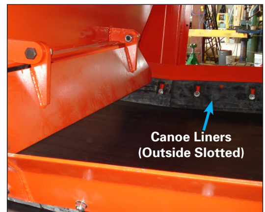
Belt Feeder with Canoe Liners on either side shown after 6 months of wear.
