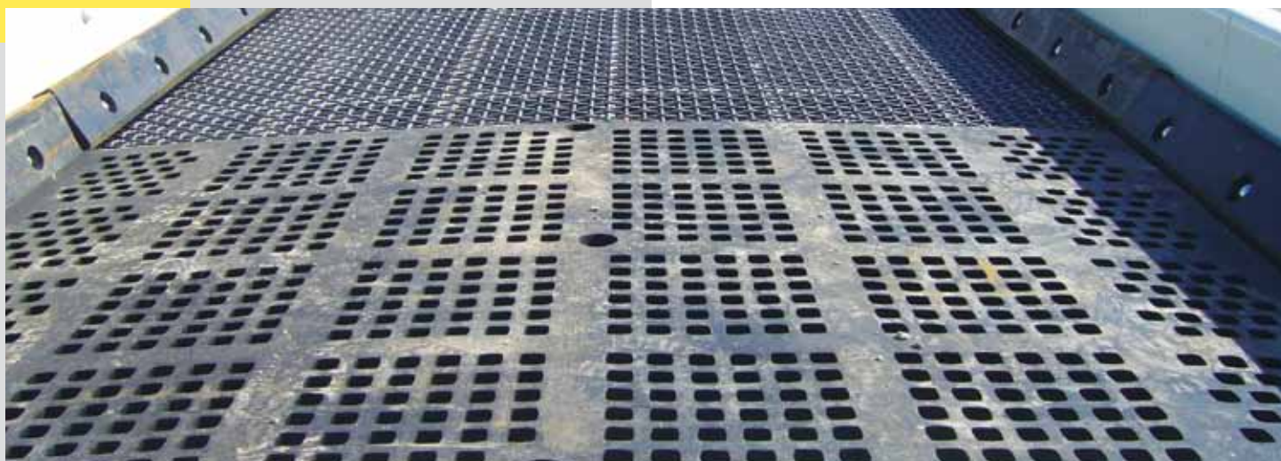
Rubber and wire cloth screen deck with rubber side tension rails
